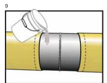
9. Reconfirm that the application temperature is above 10°C (50°F)\* & 3°C (5°F)\* above the dew point. Then slowly pour mixed epoxy onto pipe. See "Tips" below for additional suggestions.
