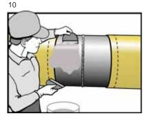
10. Use trowels, brush or roller to apply required minimum thickness of coating to the Field Joint. Cover at least 50mm (2") of the adjacent mainline coating.
