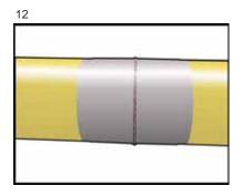
12. The curing rate\* will vary according to pipe and ambient application temperature. Refer to curing rate chart to determine when to perform a Shore D check.
