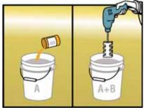
7. Warm parts A & B to 20°C (68°F) and mix by pouring all of part B into part A. Thoroughly scrape container and lid of B. Slowly begin mixing to avoid introducing air into the mixture.
