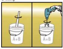
8. Use a mixing speed that uniformly blends the 2 parts, but does not create a vortex in the mixture or spillage.
