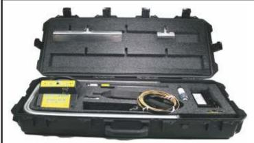
Kit includes: Instrument and Battery PowerPak and 5' Cable Ground Cable, 20' Wand and Extension Handles Battery Charger Belt Electrode\* Carrying Case Instructions
