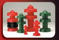
The Girard Turbo-Magnum<sup>™</sup> is a one piece, all polyurethane pig available with either 3 or 4 cups. The hollow center allows for maximum flexibility while negotiating tight radius bends and other pipeline features.
