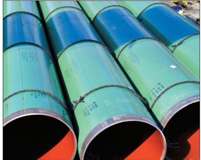
Fusion bond epoxy on American-made Dura-Bond steel energy pipe
